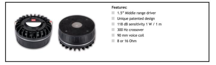
BMS 4595ND-mid is a powerful 1.5" professional compression driver that delivers outstanding sonic quality in a small package. The BMS exclusive voice coil technology employs a light weight Copper Clad Aluminium wire wound inside and outside of the Kapton™ former to improve the heat dissipation, dramatically increasing the acoustic output and reliability of the driver while minimising the power compression.
